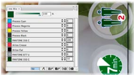
Use the full amount of available inks when making your job colors instead of only mixing the 4 process inks.
